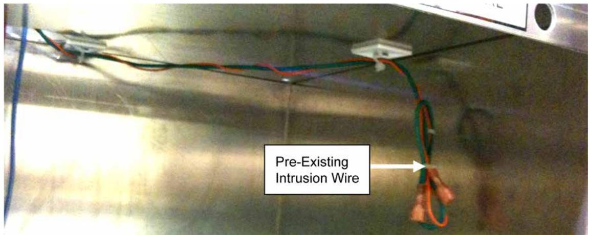
45. Install the intrusion wires from the previous step to the intrusion switch (item 10). Do this prior to installing in the cabinet.
