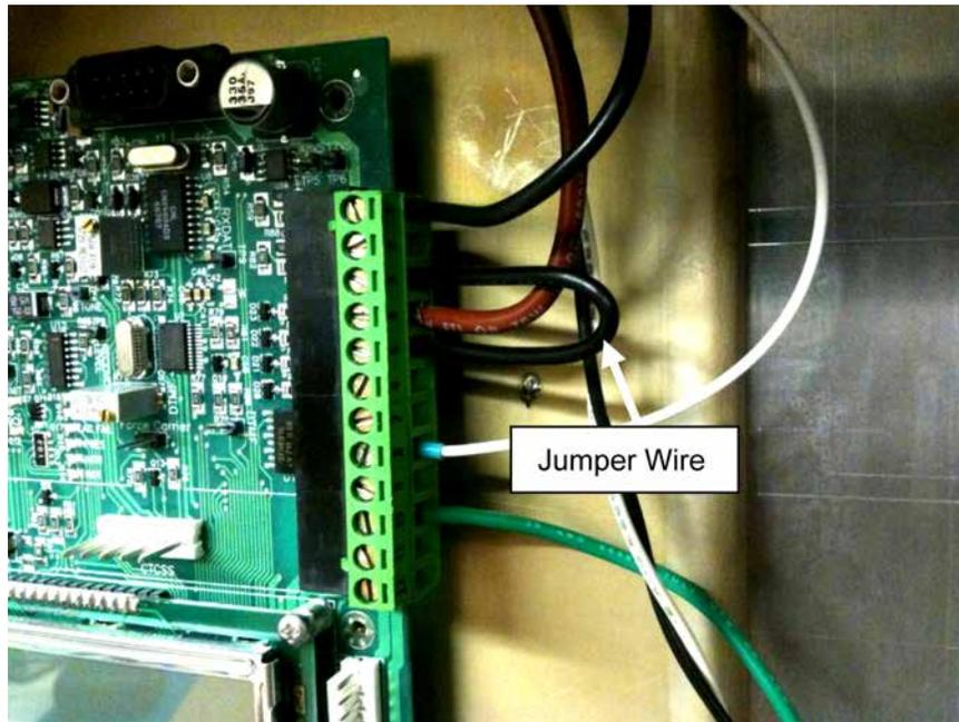
34. Install the 12 V sense wire (item 38) at the controller board. If there is any confusion, refer to schematic in the DCB, DCFCB, and DCFTB Models Manual.
