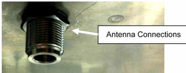
6. Ensure that all the antenna connections are sealed. If this is not sealed properly, moisture and weather may cause damage.
