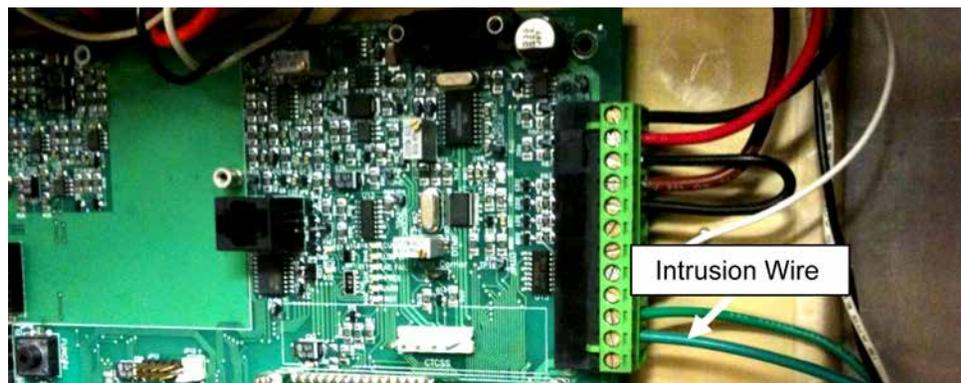
39. Install the other end of the intrusion wire to the intrusion switch. Connect to COMMON on the switch.
