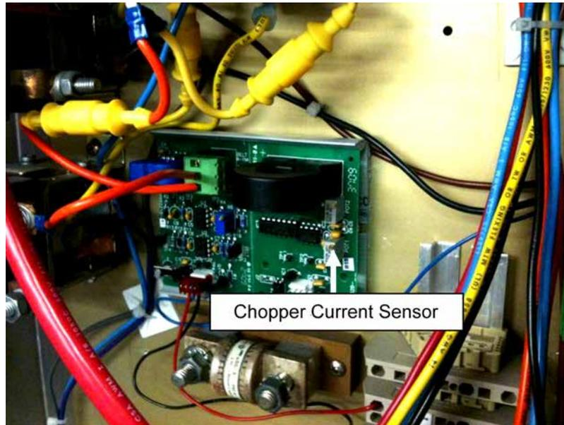
24. Connect the chopper wire assembly (item 20) to the chopper current sensor.
