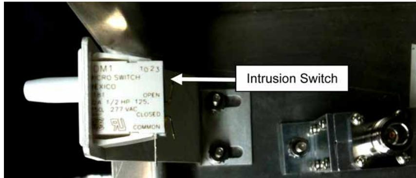
38. Install the intrusion wire (item 15) on the controller board. If there is any confusion, refer to the schematic in the DCB, DCFCB, and DCFCB Models Manual.
