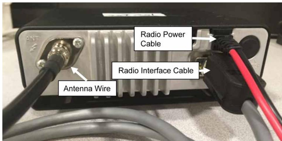
50. Connect the radio power cable (item 3) and radio interface cable (item 2) to the radio.
