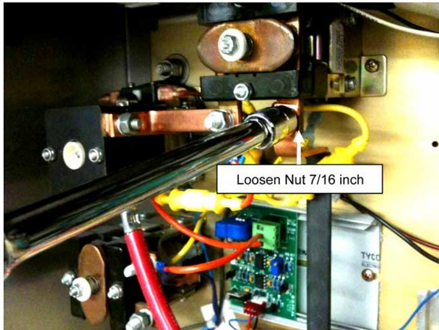
21. Loosen the nut 1/2 inch. DO NOT remove it.
