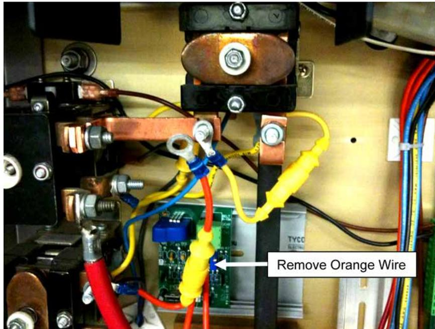
14. Connect the orange wire from the rotation current sensor. Make sure it is the one with the fuse. Reapply and tighten the nut.
