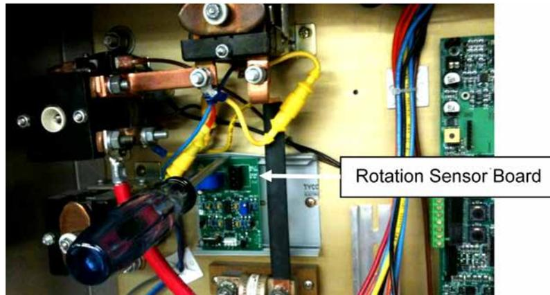
11. Plug the wire assembly (item 23) into the rotation current sensor.
