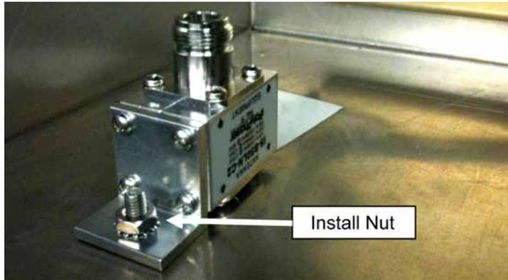
5. Connect the external antenna cable to the antenna lightning protection. The antenna was installed earlier.
