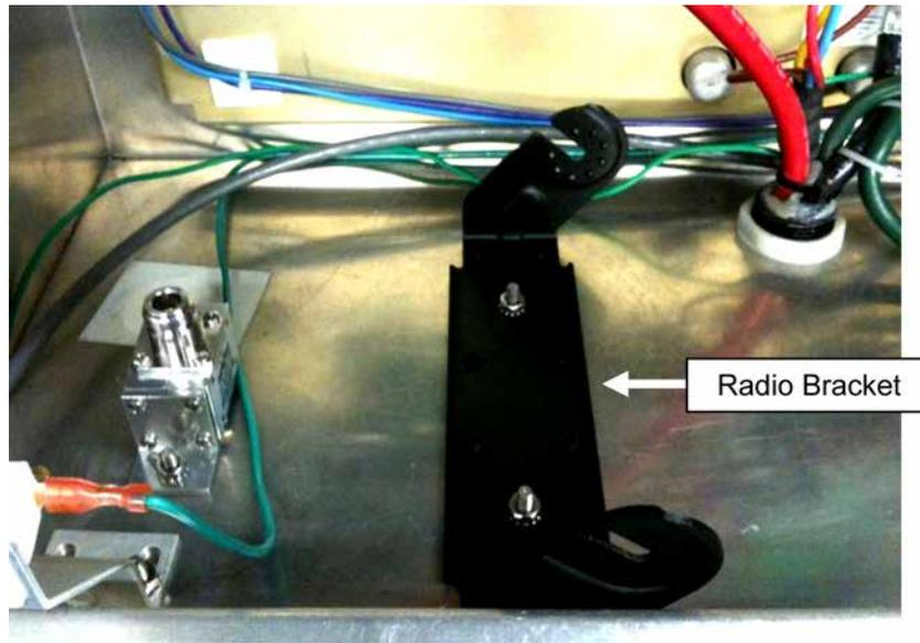
49. Connect the antenna wire (item 4) to the radio. Ensure that it is tight.
