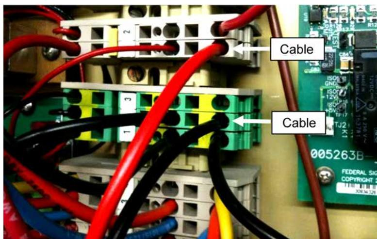
54. Connect the radio interface cable (item 2) to the controller board. Secure with screws (item 31) and the lock washer (item 34).
