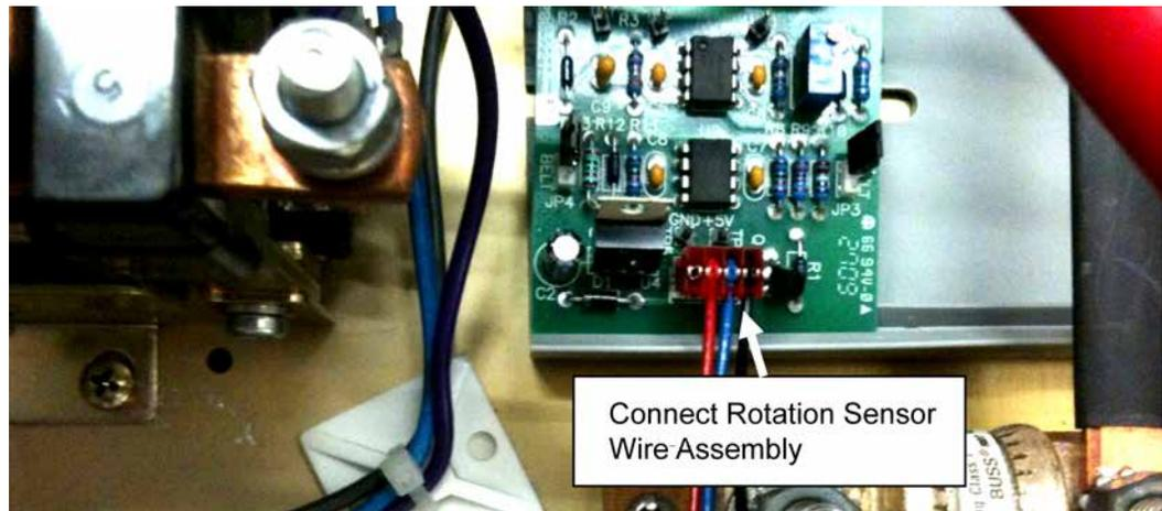
18. Connect the rotation sensor wires (item 21) to the DIN rail terminals.
