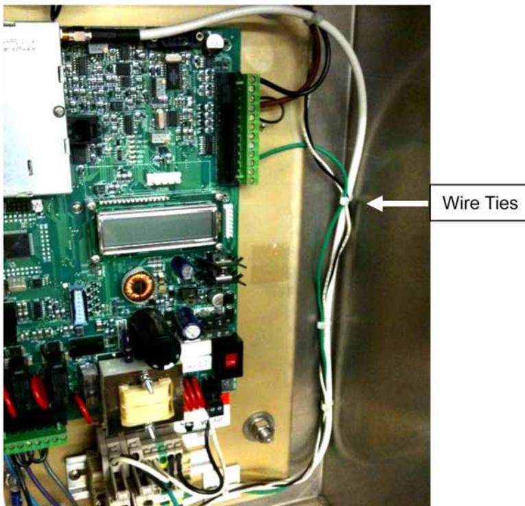
6. Remove the inside antenna cable connector from the radio.
