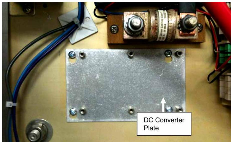
30. Install the DC converter (item 6) using screws (item 7).
