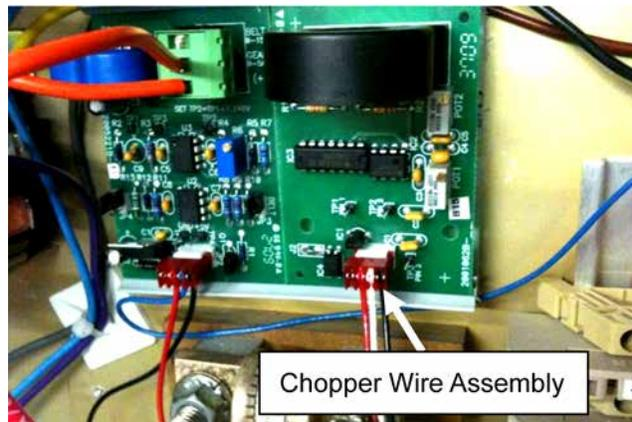
25. Connect the chopper sensor wire (item 20) to the DIN rail terminals.
