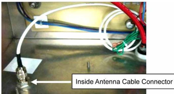
9. Remove the inside antenna cable.
