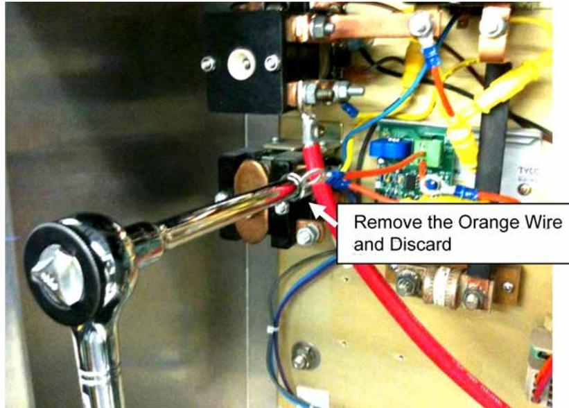
16. Connect the orange wire from the rotation current sensor. Make sure it is the wire without the fuse. Reapply and tighten the nut.
