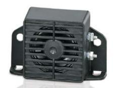
Model 252 back-up alarm is a solid state audible warning device enclosed in a weatherproof housing. The alarm produces a horn tone of 97 dBa @ 4 feet and sounds at approximately 60 times per minute with equal on and off pulses. Model 252 conforms to SAE (Society of Automotive Engineers) J994 Sound Level Type C.
