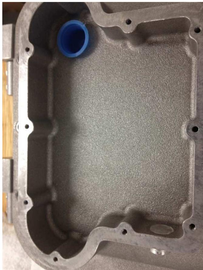
Photo 7 – No water detected in Main Enclosure
