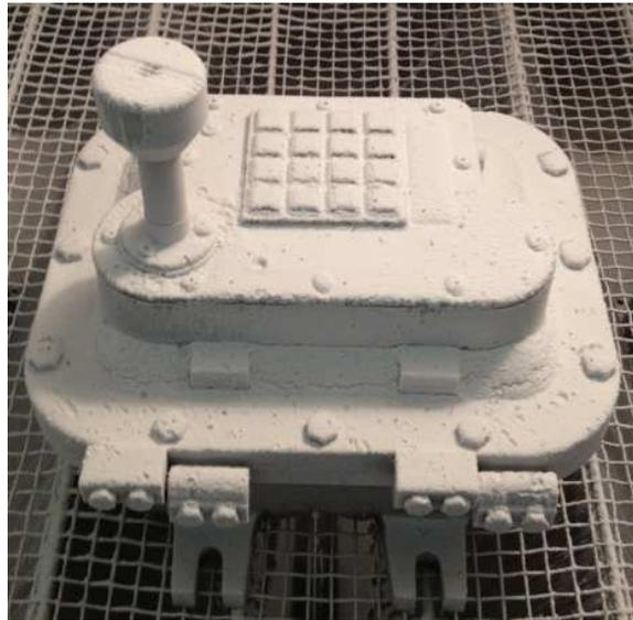
Photo 2 – No sign of talc entry at microphone
