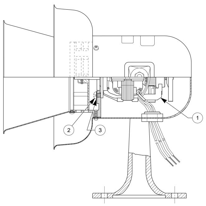
NOTE: INSTALL MOTOR IN POSITION WITH WIRES CLOSEST TO CONDUIT ENTRANCE AS ILLUSTRATED ON DRAWING.
