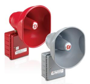
Models AM300 and AM302 are rugged, transformer coupled, re-entrant speakers for use in public address or paging applications. These 15 and 30 watt speakers feature a durable speaker cone and projector constructed of spun aluminum. The speaker wiring connections are enclosed in a dust- and moisture-proof, die-cast aluminum compartment. All external surfaces are sealed with a red or gray powder coat paint.
