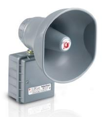
SelecTone® Model 300 is a lightweight and compact, solid-state amplified speaker designed to amplify a pre-selected tone over existing ambient noises. The speaker cone and projector are made of spun aluminum. The internal amplifier circuitry and tone module are contained in a housing of die-cast aluminum. Dust- and moisture-proof gasketing provides protection from the elements. All external components are sealed with powder-coat paint.
