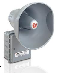
Model AM15 is a rugged, re-entrant speaker for use in public address or paging applications. This 15 watt speaker features a rugged speaker cone and projector constructed of spun aluminum. The speaker wiring connections are enclosed in a dust- and moisture-proof, die-cast aluminum compartment. All external surfaces are sealed with gray powder coat paint.
