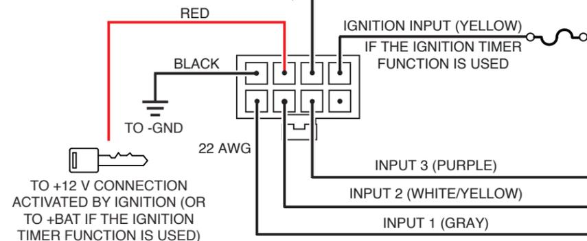
**ACTIVE-LOW INPUTS 1-4:** Ground-activated. Can be programmed to activate with the control pad, installer-supplied switches (current capacity of 100 mA each), or with the two-position switches on the steering wheel of the Ford Police Interceptor.
