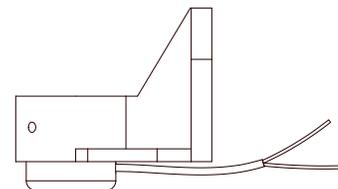
The switch is housed within a PVC holder that is mounted in the bottom steady rest bracket.
