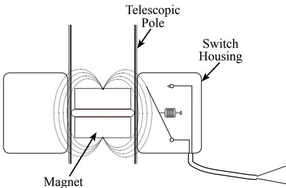
**Diagram 1. Pole Down; Magnet Holds Switch Open**
