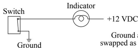
Ground and +12 VDC can be swapped as required for installation.
