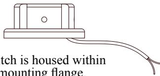
The switch is housed within the mounting flange.
