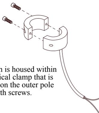
The switch is housed within a cylindrical clamp that is mounted on the outer pole with screws.
