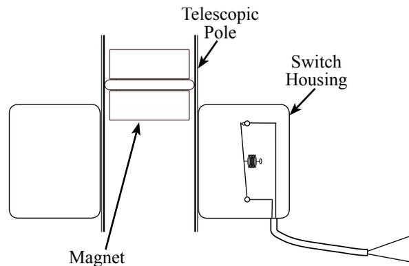
**Diagram 2. Pole Moves Up with Magnet; Switch Closes**
