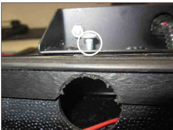
Figures 3 and 4 Drilled holes on edge of spoiler for access to #10-32 mounting kit hardware
