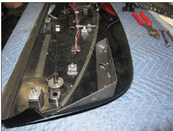
Figures 3 and 4 Drilled holes on edge of spoiler for access to #10-32 mounting kit hardware
