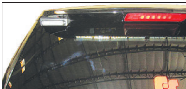
Figure 7 MicroPulse with bracket fastened to spoiler (driver side)
