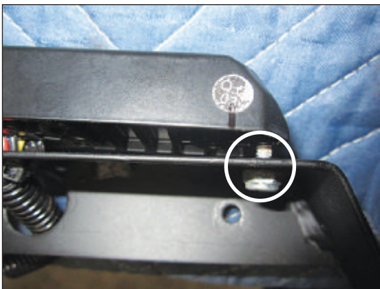
Figure 5 MicroPulse secured to bracket with #6-32 mounting kit hardware
