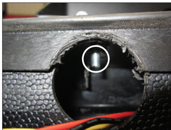
Figures 3 and 4 Drilled holes on edge of spoiler for access to #10-32 mounting kit hardware
