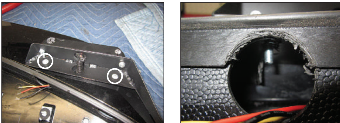
Figure 6 MicroPulse with bracket fastened to spoiler with the #10-32 hardware
