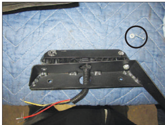
Figure 5 MicroPulse secured to bracket with #6-32 mounting kit hardware
