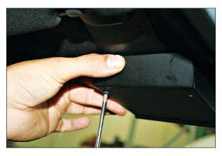
**8.** Some adjustments may be necessary to adjust the position of the visor clip bracket to ensure a proper fit to the vehicle contours. Ensure the shroud is tight against the windshield and tighten all hardware.
