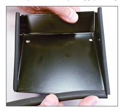
7. Make sure that you use the proper shroud (driver side or passenger side). Then position, align, and secure the shroud to the visor clip bracket with the provided #8 pan-head screws.
