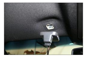
5. Place the visor clip bracket with the attached IPX6 lighthead between the visor clip and the headliner. Secure the assembly with the visor clip screw. To ensure a flush fit, it may be necessary to remove some of the extra-long plastic material surrounding the mounting hole for the visor clip (right).
