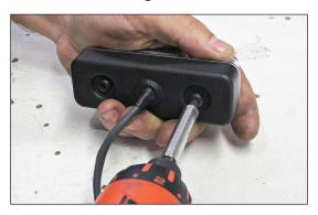
2. Install the #10-32 studs with lockwashers (supplied with the lighthead) over the long end of the stud and tighten them.
