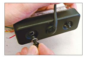
3. Place the IPX6 lighthead on the visor clip bracket as shown. Align the holes with the stude and secure them with the #10-32 KEPS nuts supplied with the lighthead.
