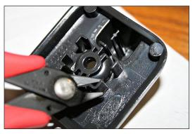
**6.** Place the sealing strip on the edges of the shroud that make contact with the windshield. Cut it to length. To hold the sealing strip in place, it may be necessary to apply a drop of "superglue" or the equivalent.
