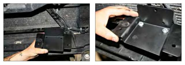
**4.** Secure the mounting bracket to the diagonal brace of the radiator support with two 1/4" x 3/4" self-drilling hex washer-head screws.
