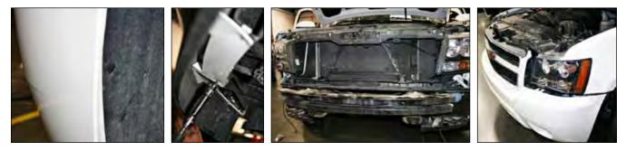
2. To make room for the speaker bracket, remove the wire-loom support fastener located on the diagonal brace of the radiator support on the driver side.
