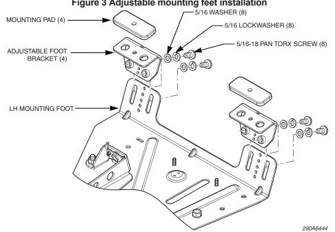
Figure 3 Adjustable mounting feet installation
