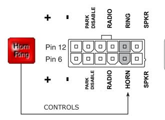
Pins 2 and 8 (gray) in the 12-pin connector on the back of the SmartSiren Platinum Siren Amplifier
