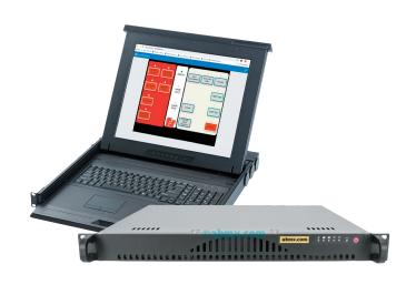
The PAGASYS GEN II System Manager Server (Model P-SERV-G) is a Windows-based server that supports the PAGASYS GEN II System Manager application to provide a user interface to the system controller.
