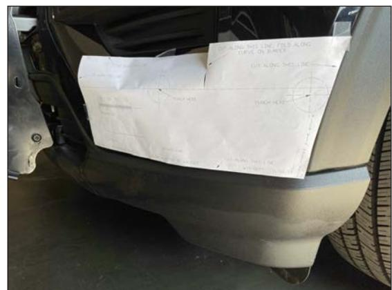
6. Using a center punch, mark the center of the two specified holes on the template. Remove the template; using a 1.5-inch hole saw, cut out the two holes and then clean the edges. See Figure 7. Repeat this process on the passenger side.
