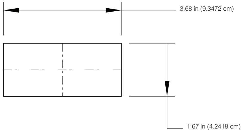
**Figure 4** Mount gasket to the back glass
