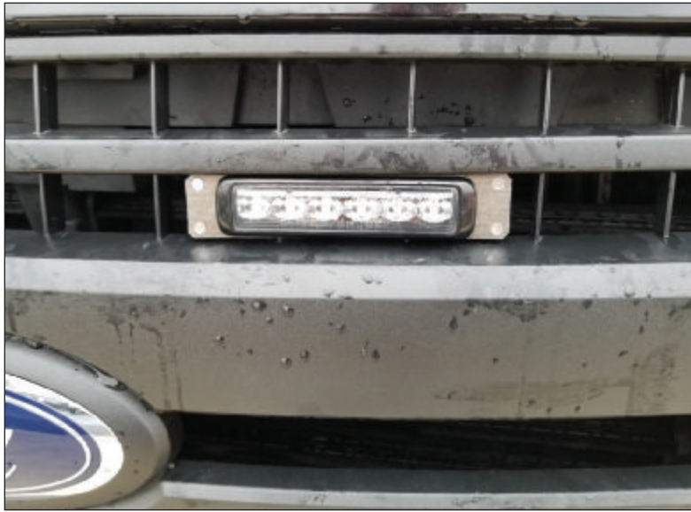
Figure 2 Brackets positioned on vertical bars on grille
