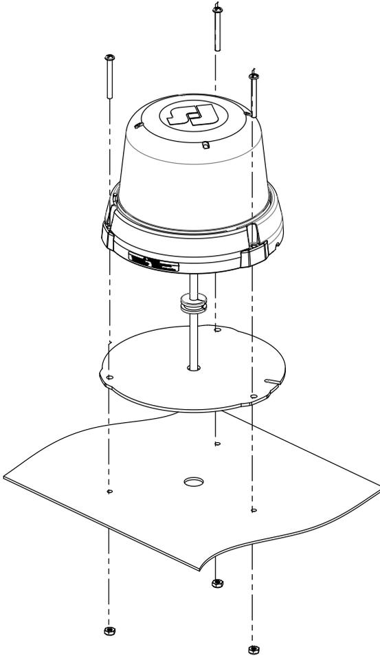
4. Align the gasket over the drilled holes. Route the wires through the gasket and wire routing hole or through the notch in the base.
