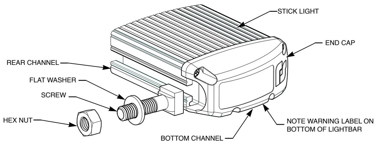
3. Drill holes as needed for the mounting screws.
