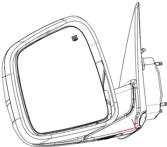
Figure 2 Final bracket position on driver-side mirror
