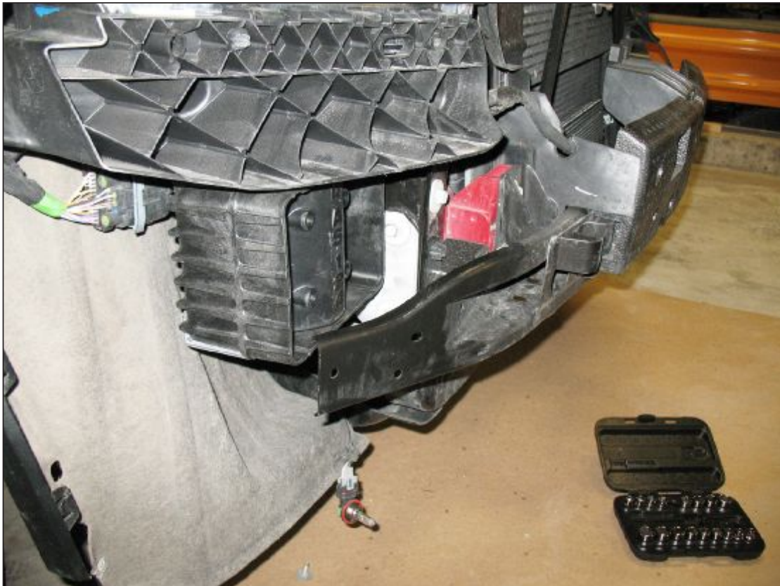
Figure 1 AS124 mounted to passenger-side core support
