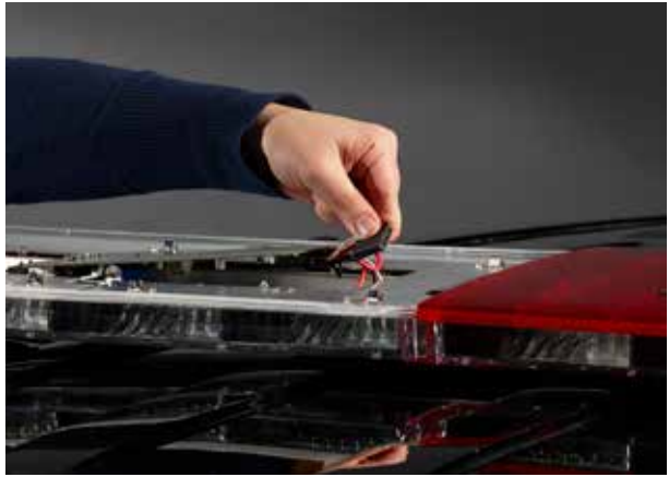
The Allegiant light bar can be serviced while on the rooftop, by removing a single dome and easily disconnecting the ROC board.
