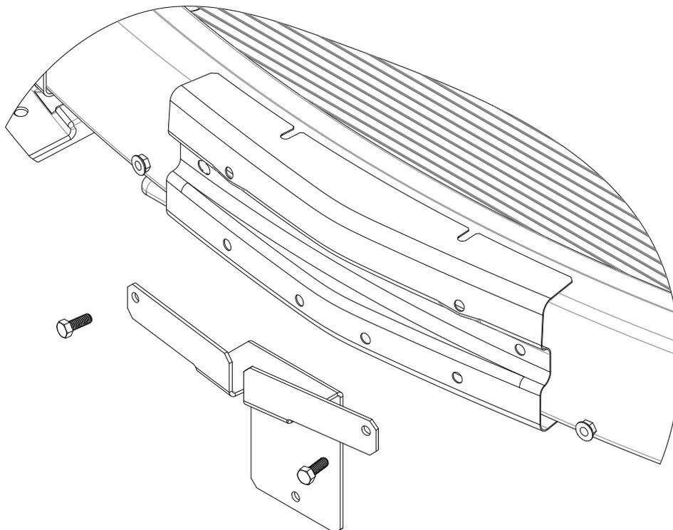
2. See Figure 1. Position the bracket over the existing holes as shown and secure with the 5/16 bolts and flanged nuts in this kit.
