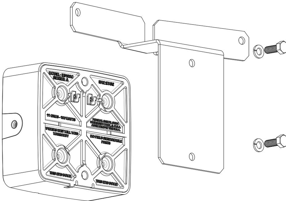
3. See Figure 2. Mount the speaker to the bracket with the 5/16 bolts and lockwashers in this kit.
