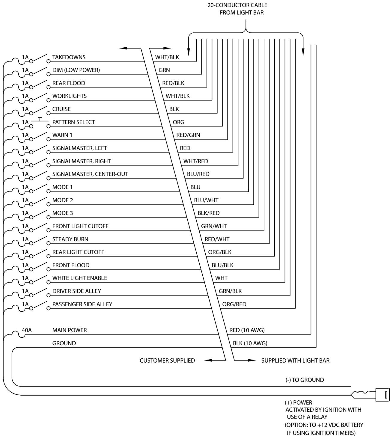
**Table 8 Light bar functions for 20-conductor cable**
