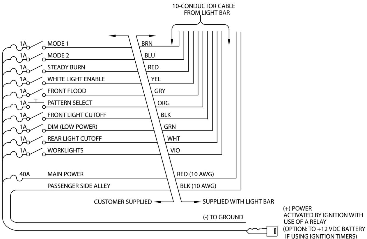
**Table 7 Light bar functions for 10-conductor cable**
