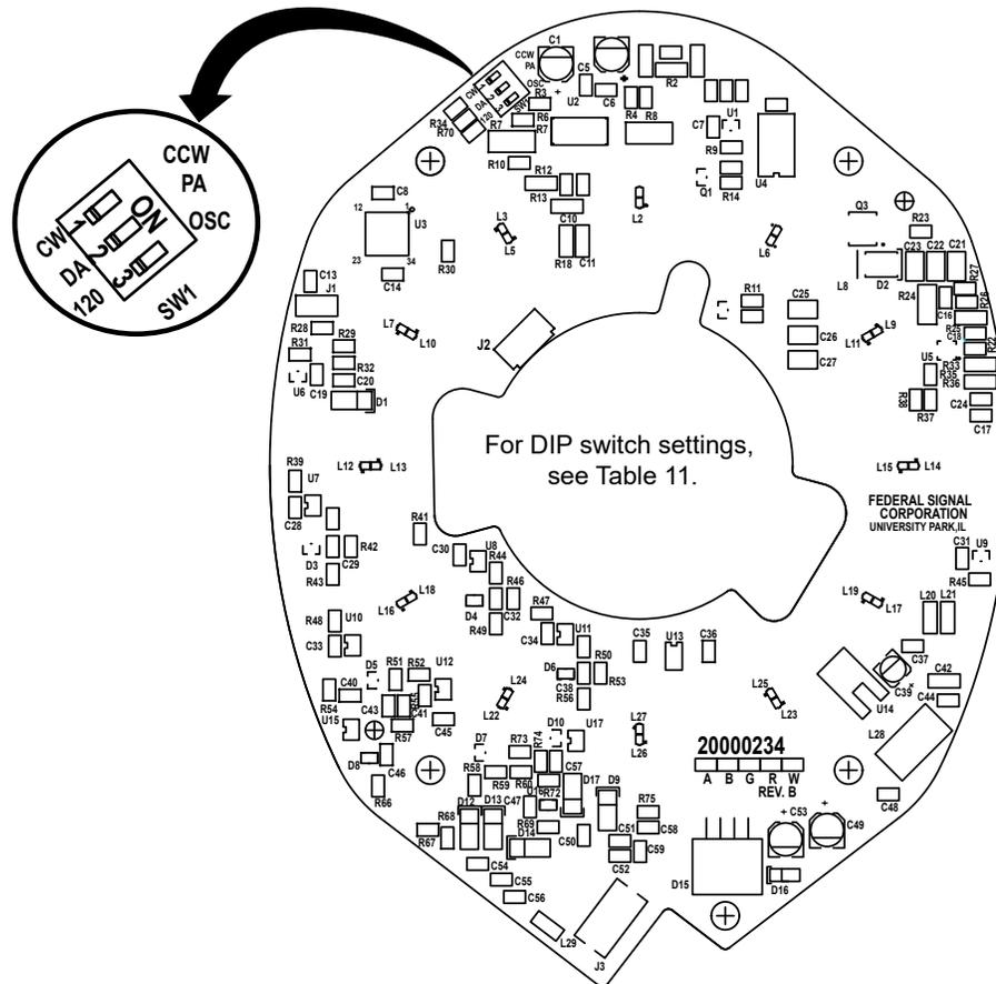
Table 11 DIP switch settings for rotator operation
