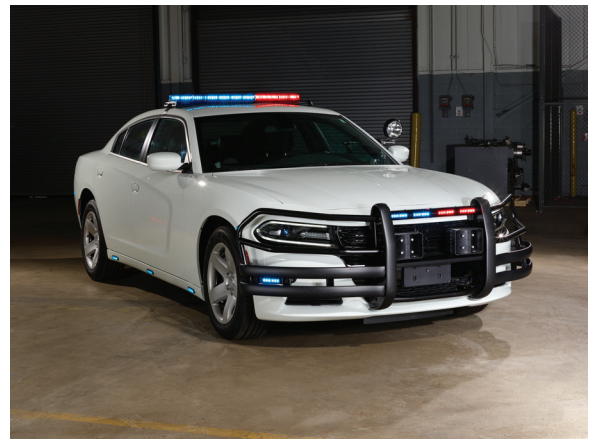
Push Bumper, Top Channel, PIT Bar and Wing Wrap shown installed on a Dodge Charger
