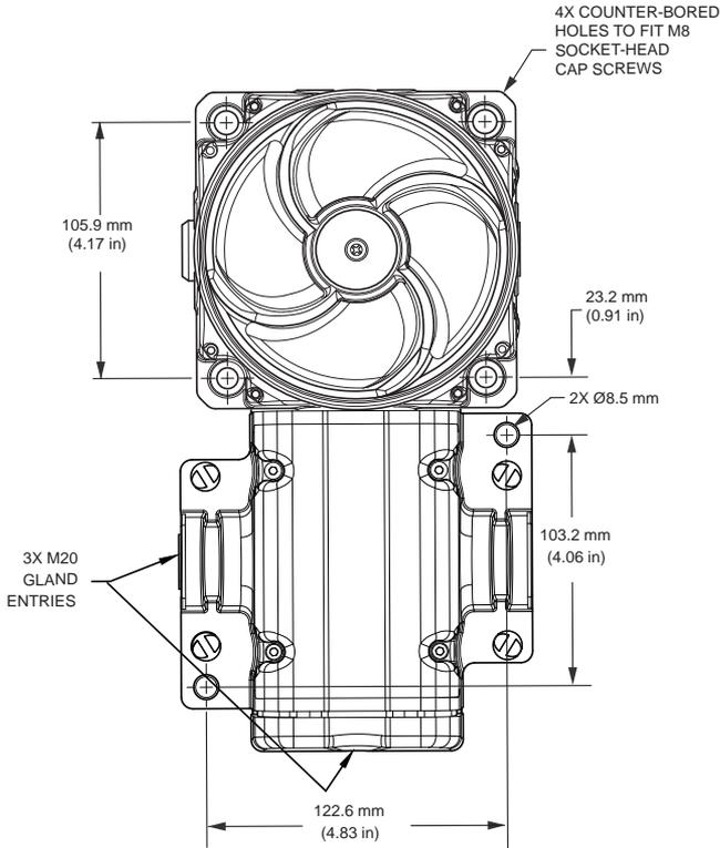
Figure 4 Side view of Ex de surface mount
