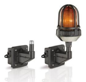
Model LHWB Hazardous Location wall mount bracket is specifically designed for use with Federal Signal's stationary warning lights to provide an easy and consistent means of securely mounting lights throughout a facility. The bracket features a 3/4-inch NPT male pipe connection. Optional bushings are available for 1/2-inch and 1 inch fixture mounting.
