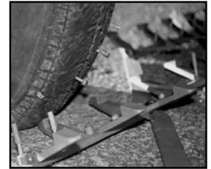
Typically, a tire picks up between four to six spikes and deflates in 12-20 seconds.
