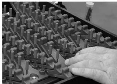
*In addition to spike replacement, check the unit for loose screws. Extend the unit fully and tighten any loose screws just enough to prevent the washer from turning. Check the rope for any knots and fraying. Also check and tighten the Quicklink of the handle to ensure it is secured properly to the base.*
