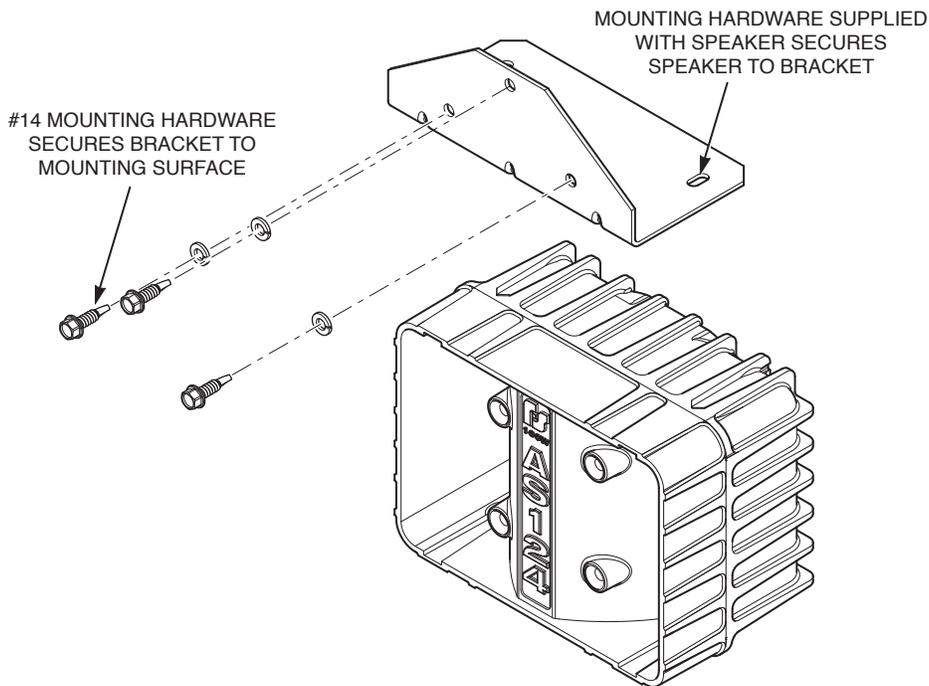
Figure 2 Speaker secured to front bumper
