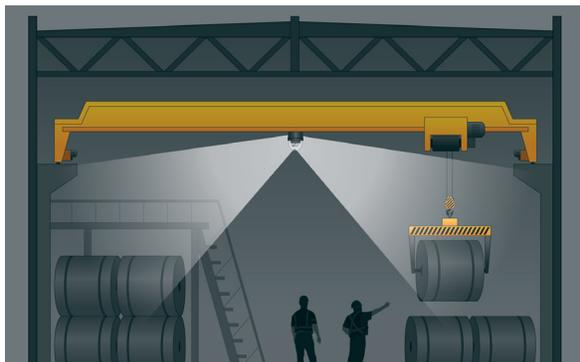
371LED/371LEDX is shipped from the factory with the standard reflector that creates a horizontal light beam that is 90 degrees from the vertical orientation resulting in a wide light output distribution.
