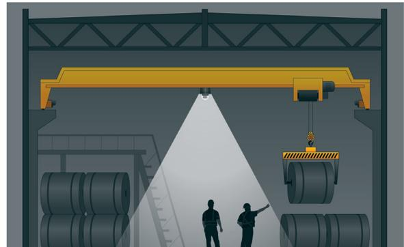
371LEDX with the 371LED-KIT-CR reflector installed reflects the light beam at 22.5 degrees from the vertical orientation resulting in a focused light output.
