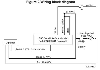
**NOTE:** Powering multiple devices with a common control lead may cause one or more units to briefly remain functional after signal power is removed. For example, due to the high input filter capacitance, a strobe supply can briefly supply the current required to signal a light bar function to remain ON. If necessary, use a relay to isolate devices with large filter capacitors. See Figure 3 for the schematic.
