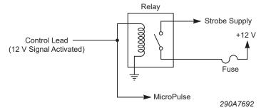
To activate a mode, apply 12 Vdc to a MODE control lead. There are three prioritized modes of operation available, with MODE 3 as the highest priority. MODE 3 overrides MODE 2, and MODE 2 overrides MODE 1. One of the available flash patterns can be programmed to each mode input. To program a flash pattern, use the Convergence Network Configuration Software.
