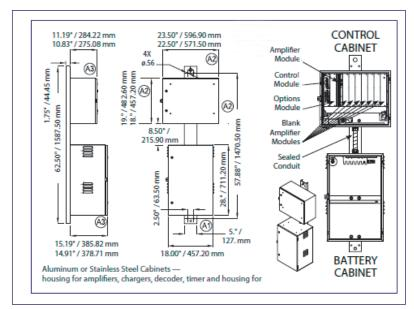
Operating Temperature \*\*: -40°F to 149°F / -40°C to 65°C Input Voltage: 120/240VAC ±10%, 50/60Hz single-phase (two separate models)
