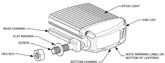
Figure 1 Stick light positioned horizontally with mounting hardware
