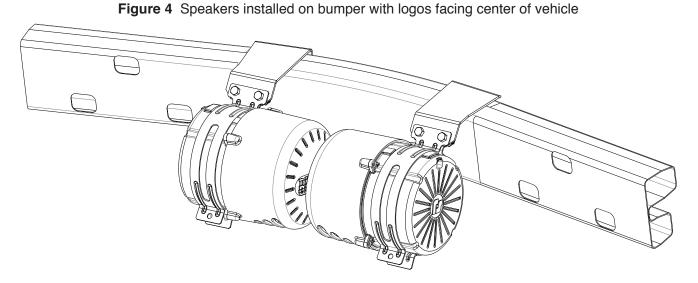
**8.** After you mount the speakers, connect the supplied wire harness to the leads from the amplifier. For details, refer to the instructions included with the amplifier.
