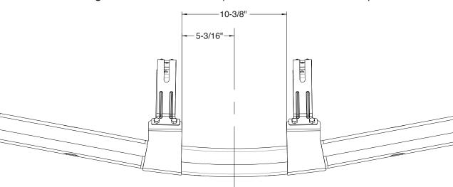
Figure 3 Distances between speakers relative to center of bumper
