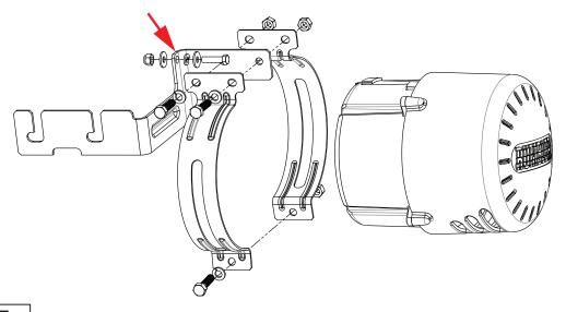
Figure 2 Driver Side Rumbler and Bracket Assembly
