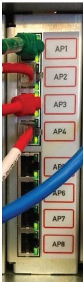
**Figure 42 External AP Mux Card Connections**
