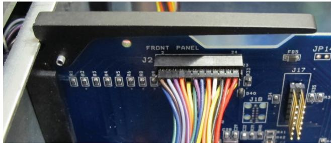
4. Unplug the fan cable near the front fan.
