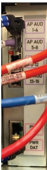
10. Plug the cables from the Access Panels or Access Panel Aggregator card into the RJ45 jack sockets located on the card installed in the AP Mux slot 2.
