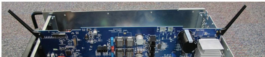
8. Holding by the open handles, carefully slide the card out of the chassis.
