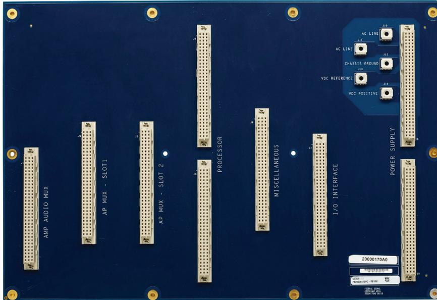
Table 3 lists the PAGASYS GEN II controller cards that can be inserted into the backplane.
