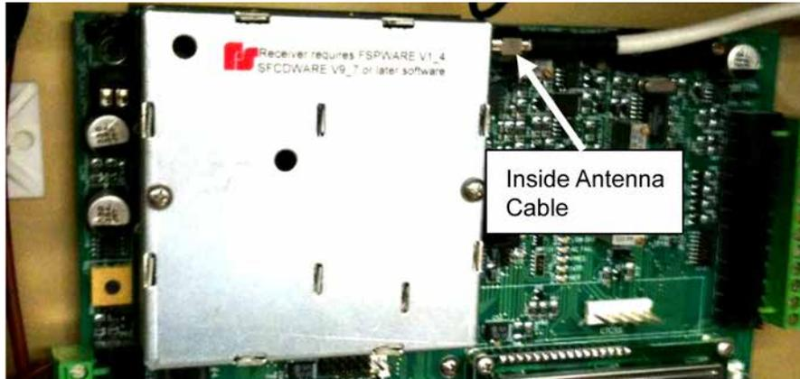
7. After removing the two screws, remove the radio by pulling the radio away from the board.
