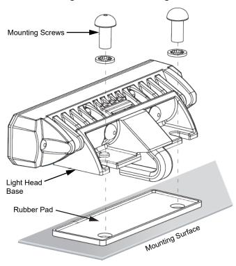
**Figure 3 Screw Mounting**
