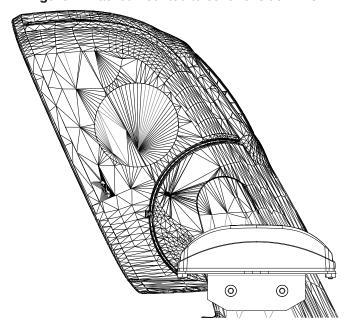
Figure 1 Bracket mounted to cover of side mirror
