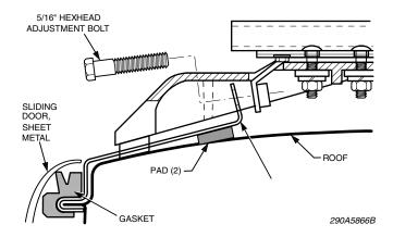
Figure 1: Lightbar attached to vehicle with hook kit
