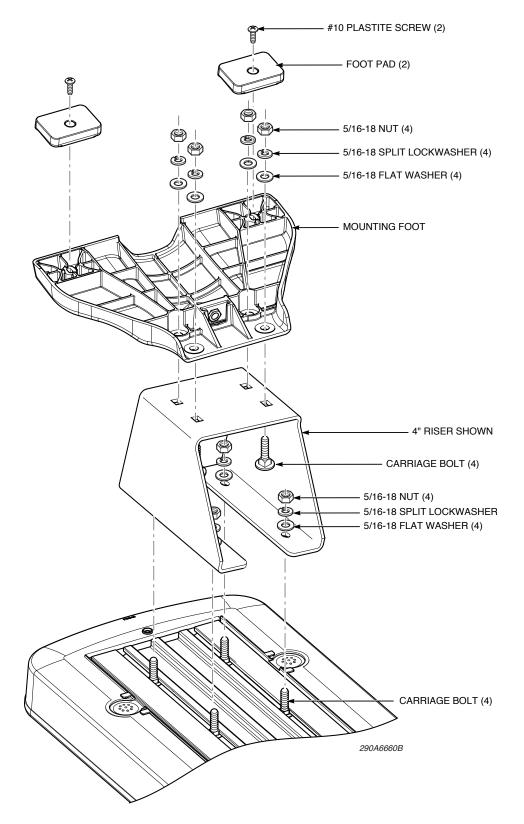
Figure 1 Mounting foot and riser bracket secured to lightbar
