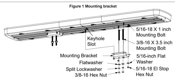
**5.** Attach the light bar to the mounting surface using the 3/8-inch hardware.
