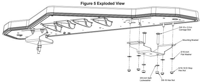
6. Attach the light bar to the mounting surface using the 3/8-inch hardware.
