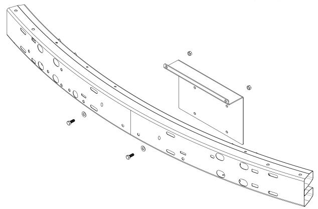
Figure 2 Exploded view of ESB2-CHGR15 bracket kit installed on Dodge Charger
