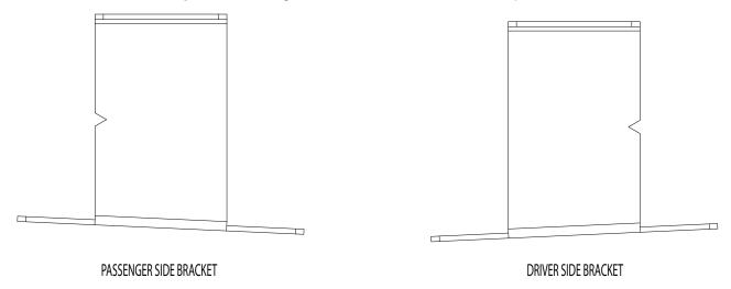
**4.** Place the driver side bracket on the grille in the location shown in Figure 3. It is necessary to insert the bracket through the center opening in the grille to allow the bracket to fit.
