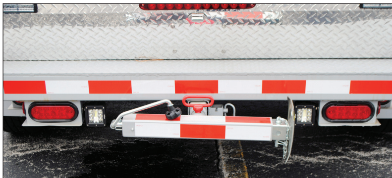
Figure 77 Back outrigger (#6) in the stowed position
