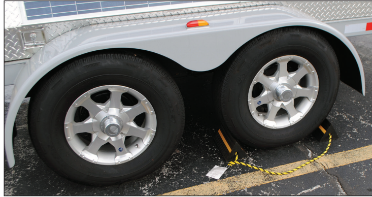
Figure 19 Wheel chocks in front and back of the tire
