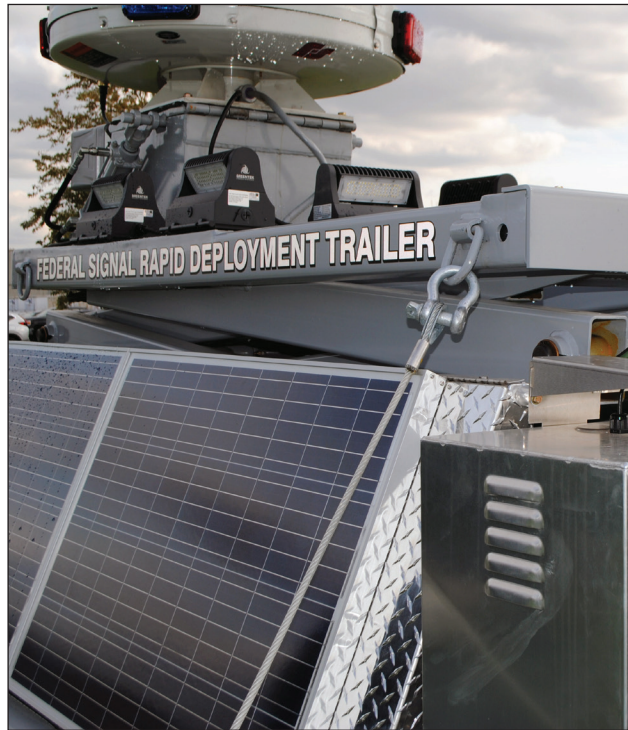
Figure 52 D-rings with a shackle attached
