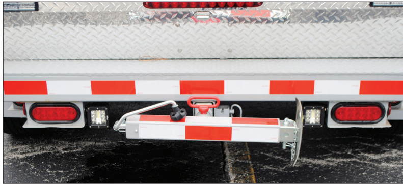
Figure 33 Back outrigger (#6) in the stowed position
