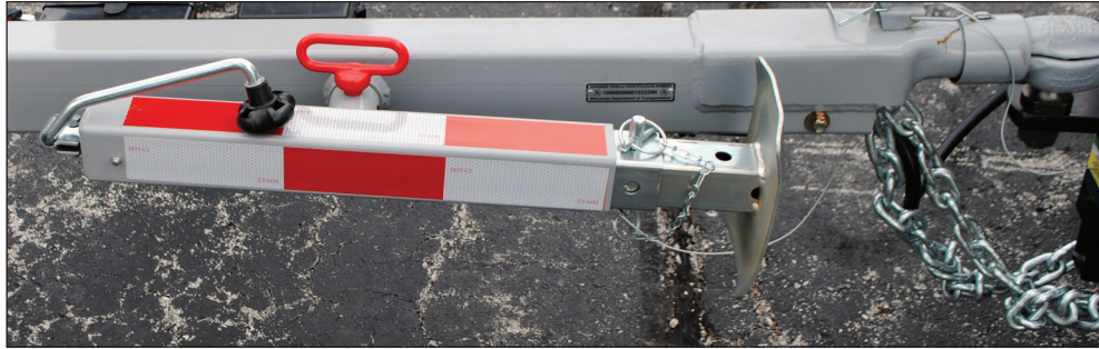
Figure 15 Front outrigger in the stowed position
