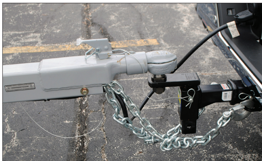
Figure 14 Breakaway cable connected to the tow vehicle
