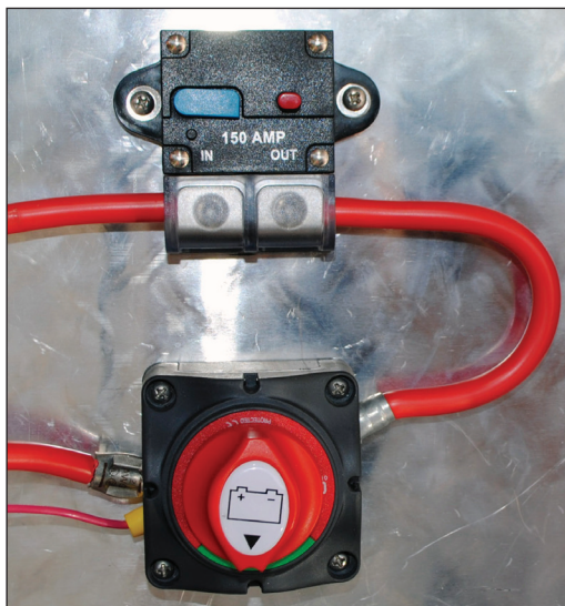
Figure 40 Main battery switch in ON position
