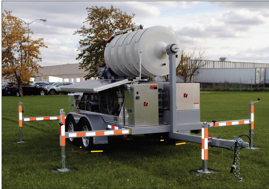
Figure 39 Outriggers deployed on a grass surface
