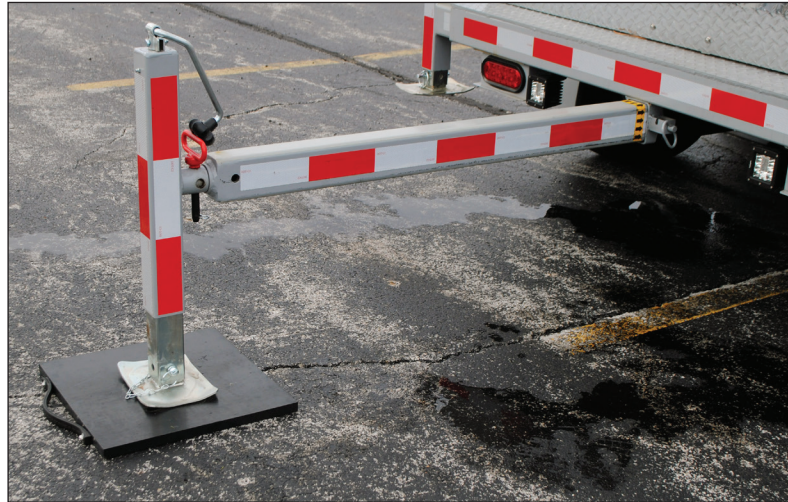
Figure 37 Support pad under outrigger #6
