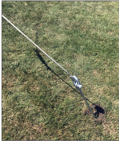
Figure 57 Cable attached to the ground anchor
