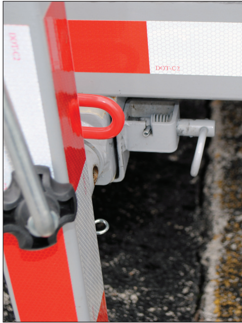
Figure 35 Spring-loaded safety latch rotated
