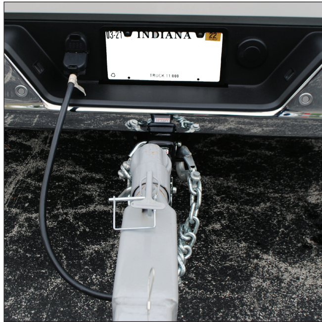
Figure 13 Multi-pin electrical connector connected to the tow vehicle
