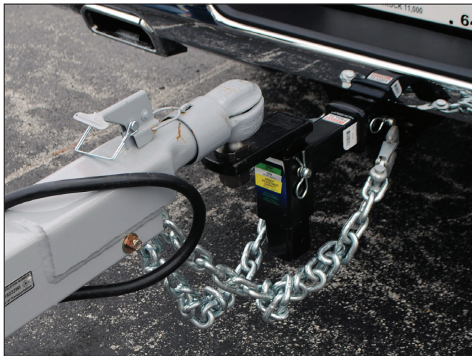
Figure 12 Safety chains attached to the tow vehicle
