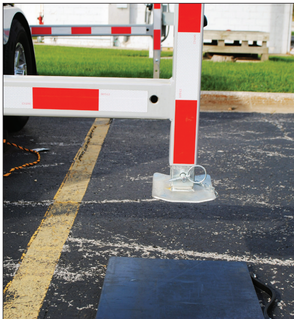
Figure 28 Locking pin unhooked
