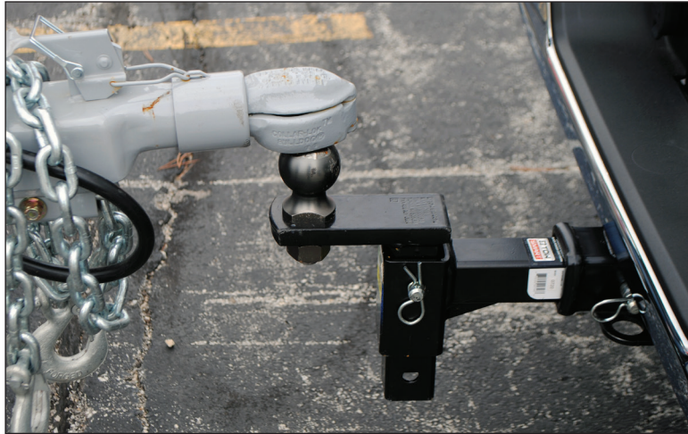
Figure 10 Trailer ball under the coupler
