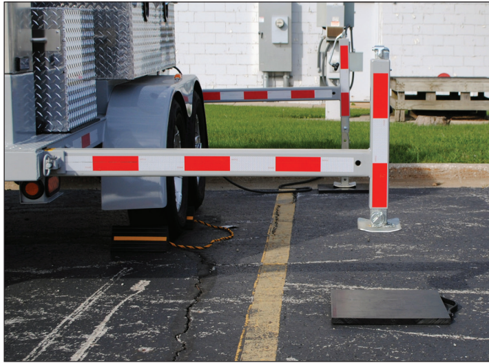
Figure 27 Support pad under the outrigger
