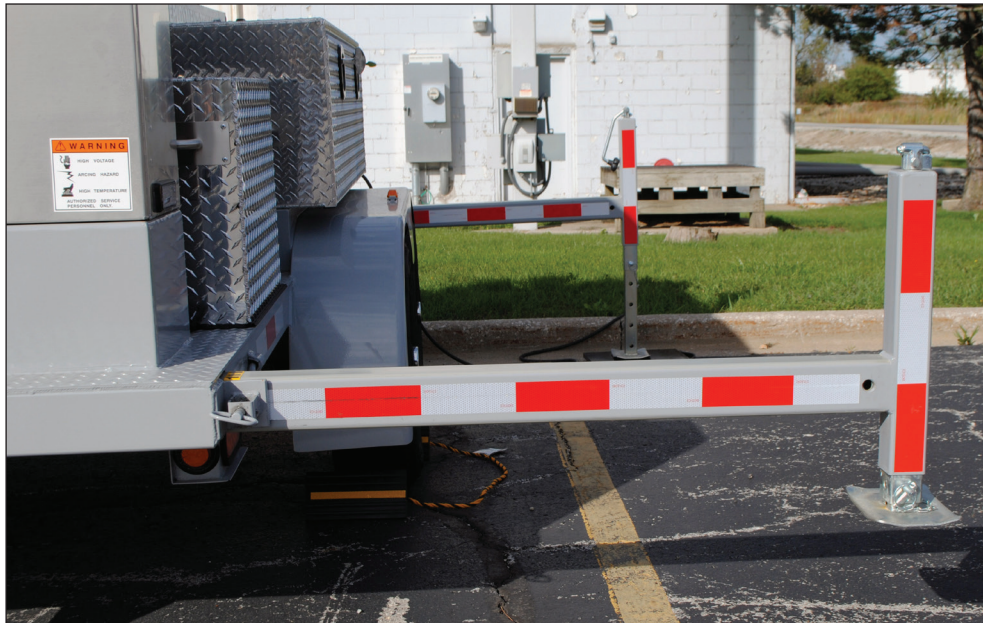
Figure 24 Pull outrigger outward to the marked stopping point
