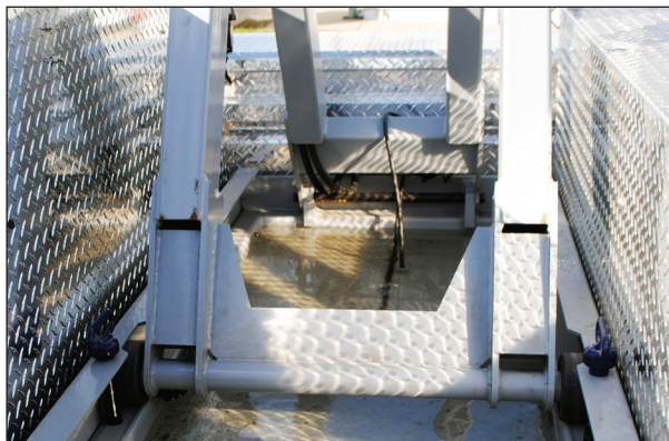
Figure 68 Locking pins in place (remove passenger's side first)
