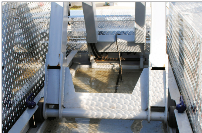
Figure 59 Locking pins in place
