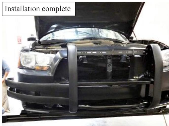
17. Align and adjust the pit bars and push bar as necessary then tighten and torque all remaining fasteners:
