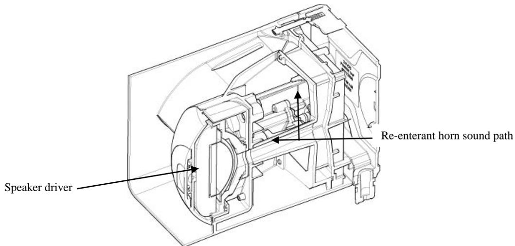
Fig 5: Electronic Horn and Siren utilizes speaker driver and reentrant horn
