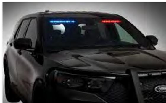
SpectraLux® ILS Low Profile SIFMJ installed on a Ford Police interceptor Utility, 2020
