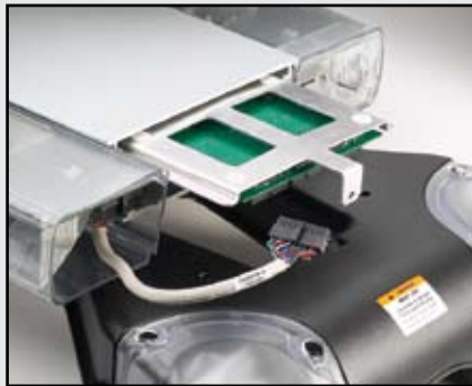
ROC with the Micro-processor Controller provides advanced communication between the lightbar and the controller head.
